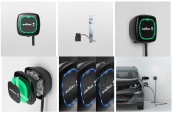
anywhere. Its dimensions are 16,6 x 16,3 x 8,2 cm and it only weighs 1 kilo (both figures excluding the hose). It incorporates an LED indicator that reflects the charging status through an intuitive code. In addition, it is extremely durable thanks to its IP54 water resistance, IK08 shock resistance and electrical protection provided by DC 6 mA leak detection.
